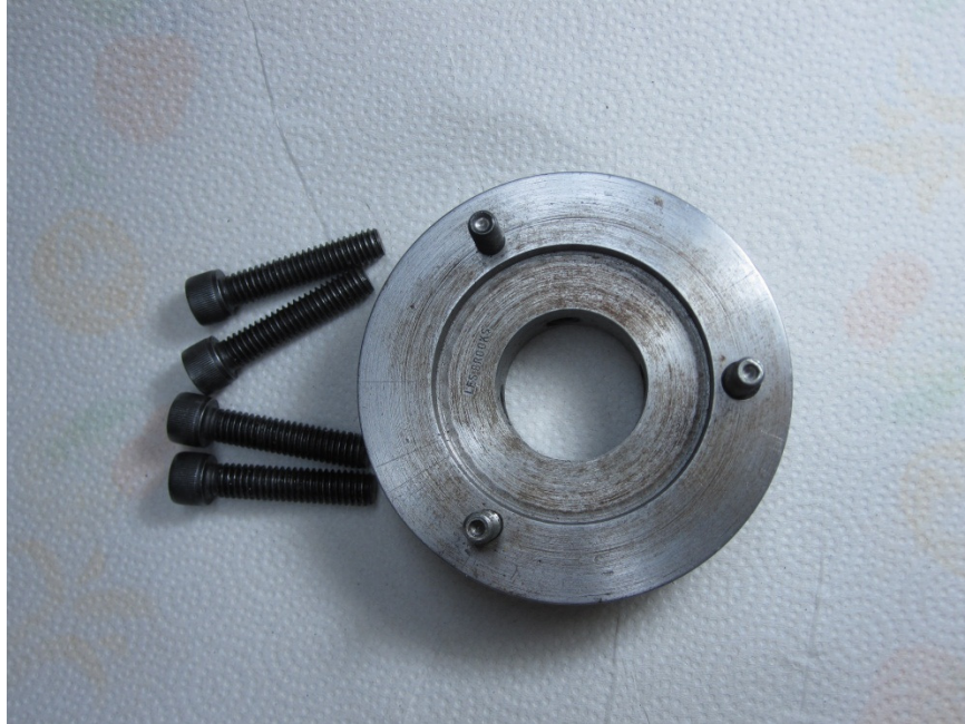
Inside cut to fit on spindle .125 Deep Spindle dia. 2.165
