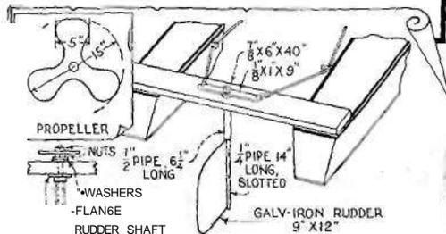
the fitting on the shaft, while the latter runs through a bearing provided directly under the rear angle-iron crosspiece. This bearing and its hanger are made up of pipe fittings as shown in Fig. 11.
